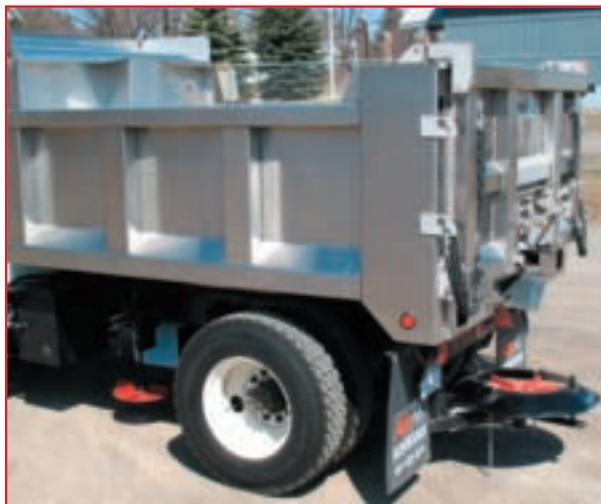
When spreading, the Flo'N Dump UNI-BODY has the lowest center of gravity of any multi-purpose body. A lower center of gravity makes the Uni-Body stable and safe on icy winter roads.
