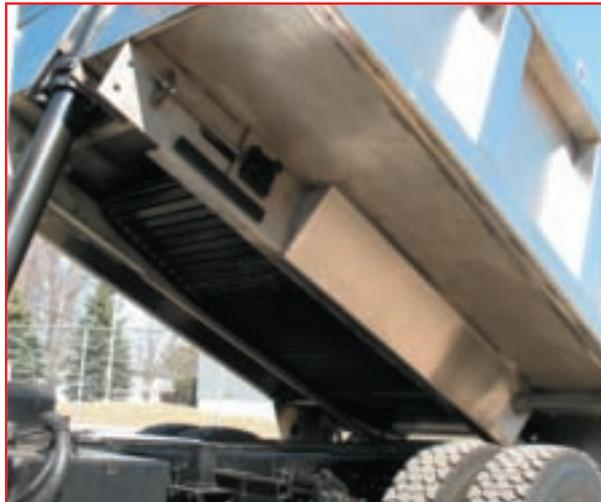
The conveyor combined with the trapezoidal longitudinals and a crossmemberless AR-400 floor, make for a very strong, efficient, and low maintenance multi-purpose dump body.
